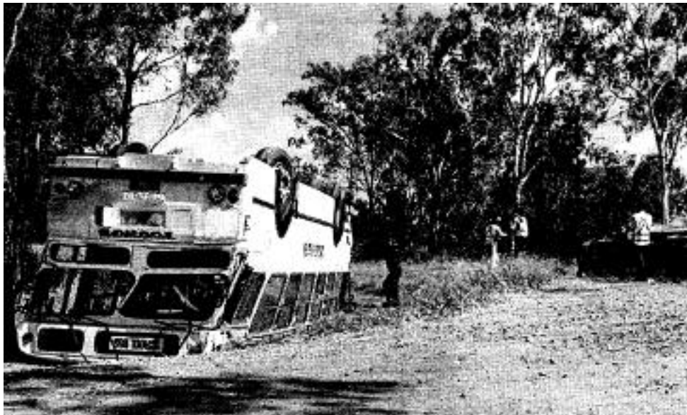
Figure 2. Deformation of Roof Structure on Rollover.
